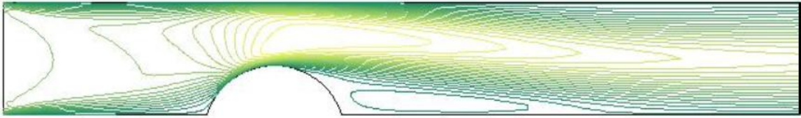
Figure 1.1: Illustration of complex flow pattern through a stenotic vessel. Typically, shear stress is very high at the throat and very low in regions of recirculation immediately after the stenosis.
