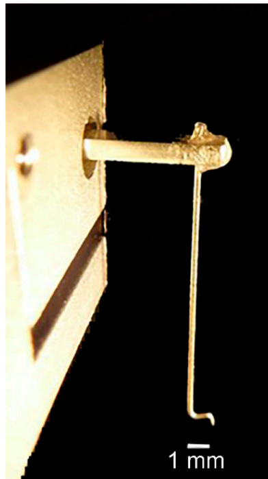
Figure 4. Force transducer “L”-shaped pin design: This pin rests on the bump on the dactylopodite and relays the force to the transducer as the cheliped opens with stimulation.
