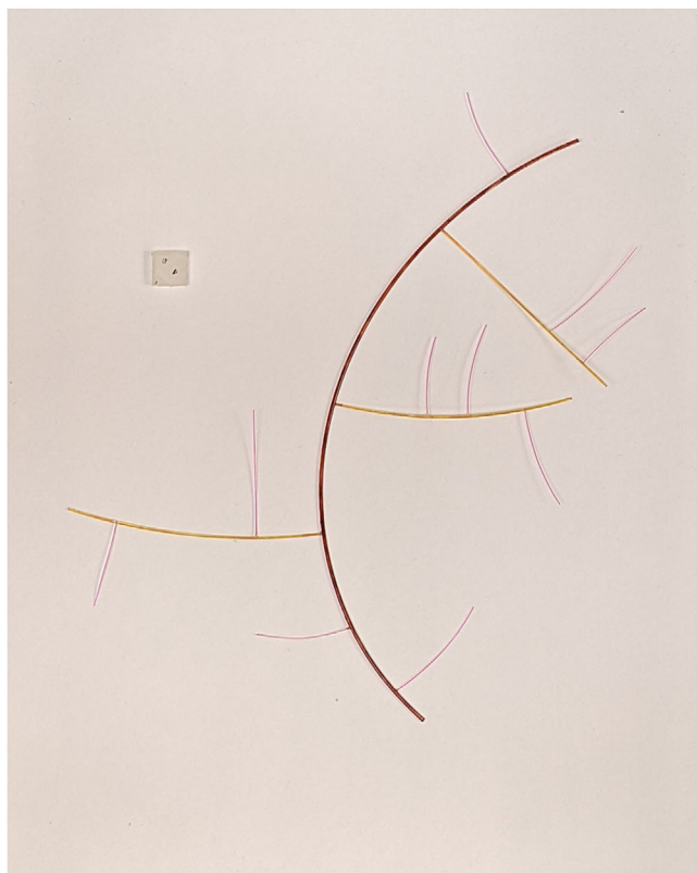
FIGURE 5 An example of a monofilament root model photographed against a white cloth background. Pink filament has a diameter of 0.3 mm, tan filament has a diameter of 0.7 mm, and the dark brown filament has a diameter of 1.2 mm. Plastic chip is 1 cm × 1 cm
