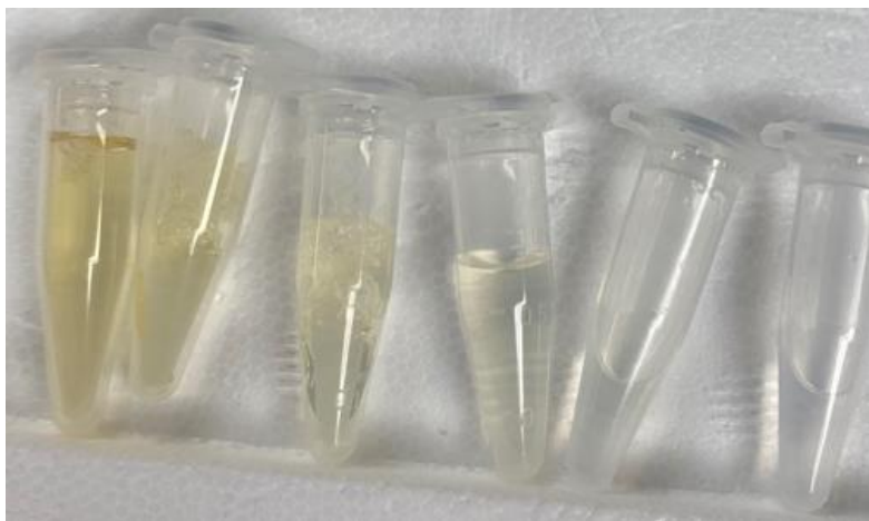
Figure 5.1 DEGDA/TTD gels with 45, 30, 20, 10, 5 and 1 monomer feed wt% (left to right).
