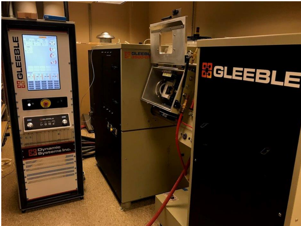
Figure 8-2 Gleeble 3500 Thermomechanical Simulator (photograph courtesy of Alyssa Stubbers).
