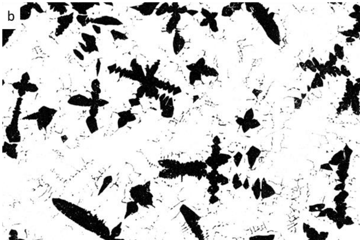
Figure E-1 (a) SE micrograph of WMoFeNi (b) threshold tool in Image J to show W dendrites in black and the rest in white.
