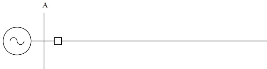
Figure 2 - One Line Diagram of Transmission Radial Line
