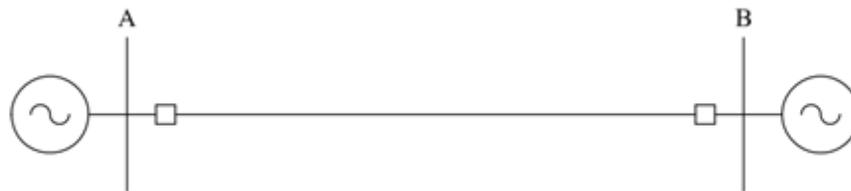
Figure 3 - One Line Diagram of Two-Terminal Single Transmission Line
