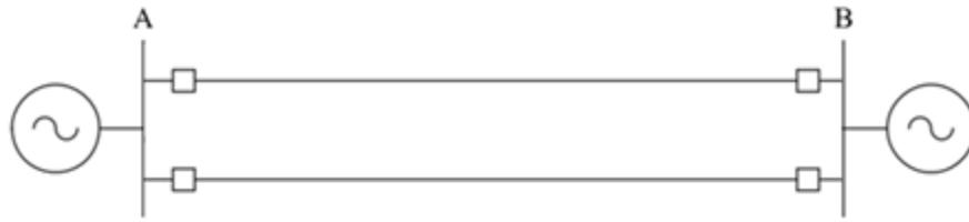
Figure 4 - One Line Diagram of Two-Terminal Parallel Transmission Line
