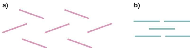
Figure 1.3: Simple representations of (a) herringbone and (b) brickwork packing motifs.
