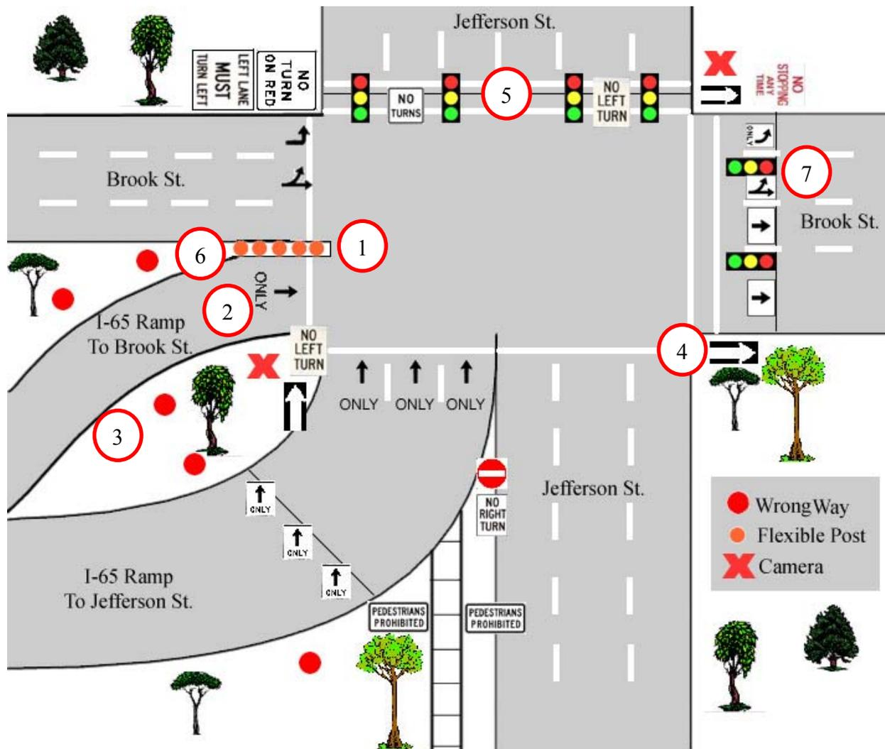
Figure 4. AIRS signage and traffic control (trees not representative of actual locations).
