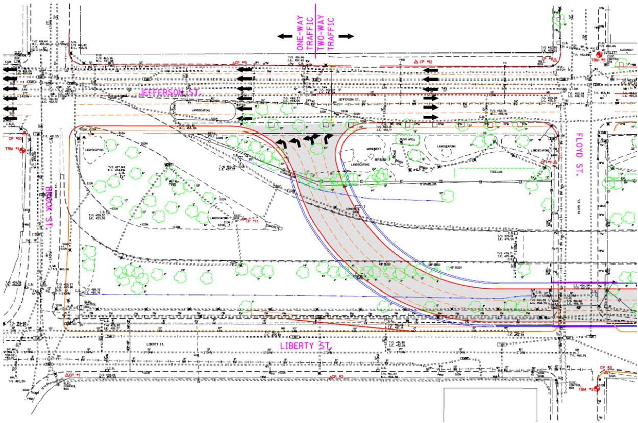
Figure 5. Brook and Jefferson intersection redesign. Shaded roadway represents the new alignment.
