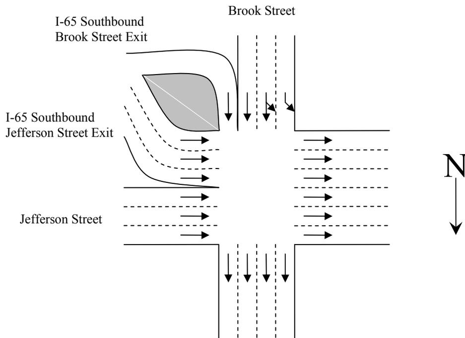
Figure 2. Intersection lane assignment
