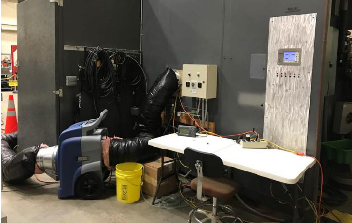
Figure 3.3: Environmental Chamber and Dehumidifier Controls [23]
