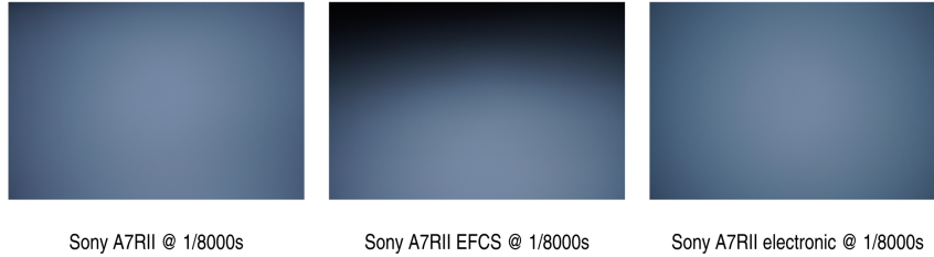
Figure 3.4: An image from a Sony A7RII illustrating the effects of the different shutter regimes.
