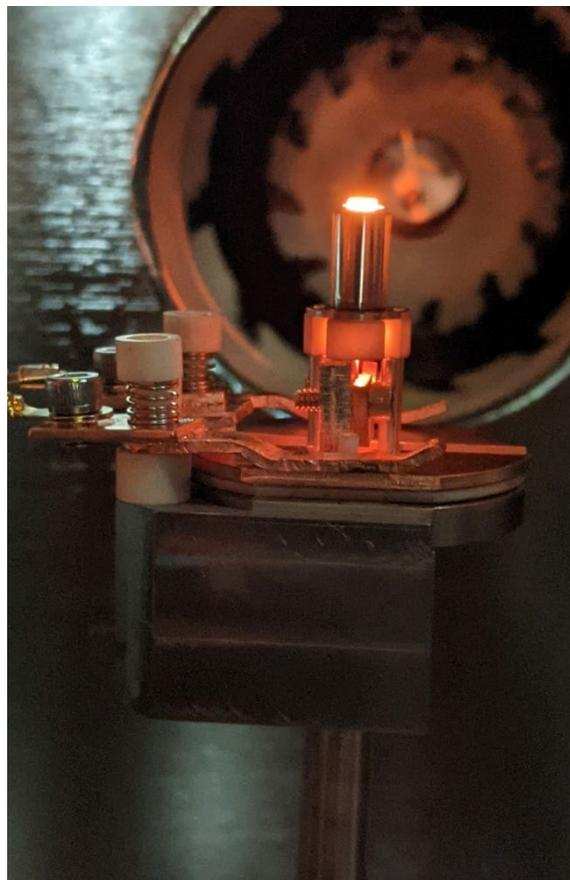
Figure 2. A red-hot glowing cathode mounted on the heating assembly of the CCC viewed in profile.
