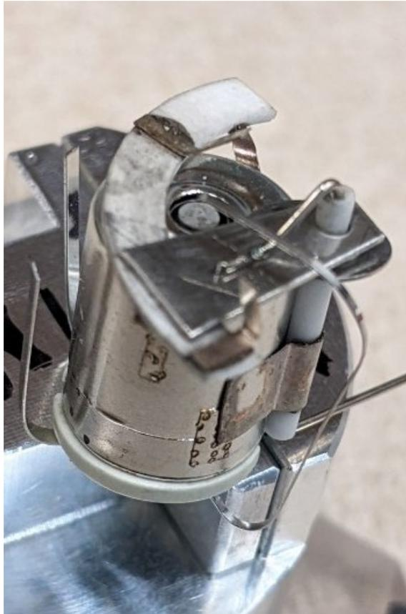
Figure 34. Custom UHV CSD assembly. Built by eBeam Incorporated. The ~2 mm diameter cathode face can be seen, as the anode plate is swiveled downward in an open position.
