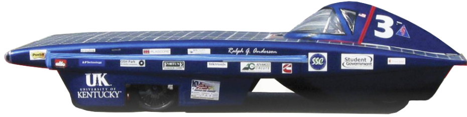
Figure 3.1: Gato del Sol IV solar car from University of Kentucky.
