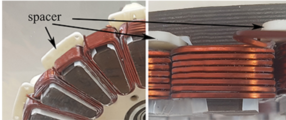
Figure 2.25: The prototype machine with spacers.
