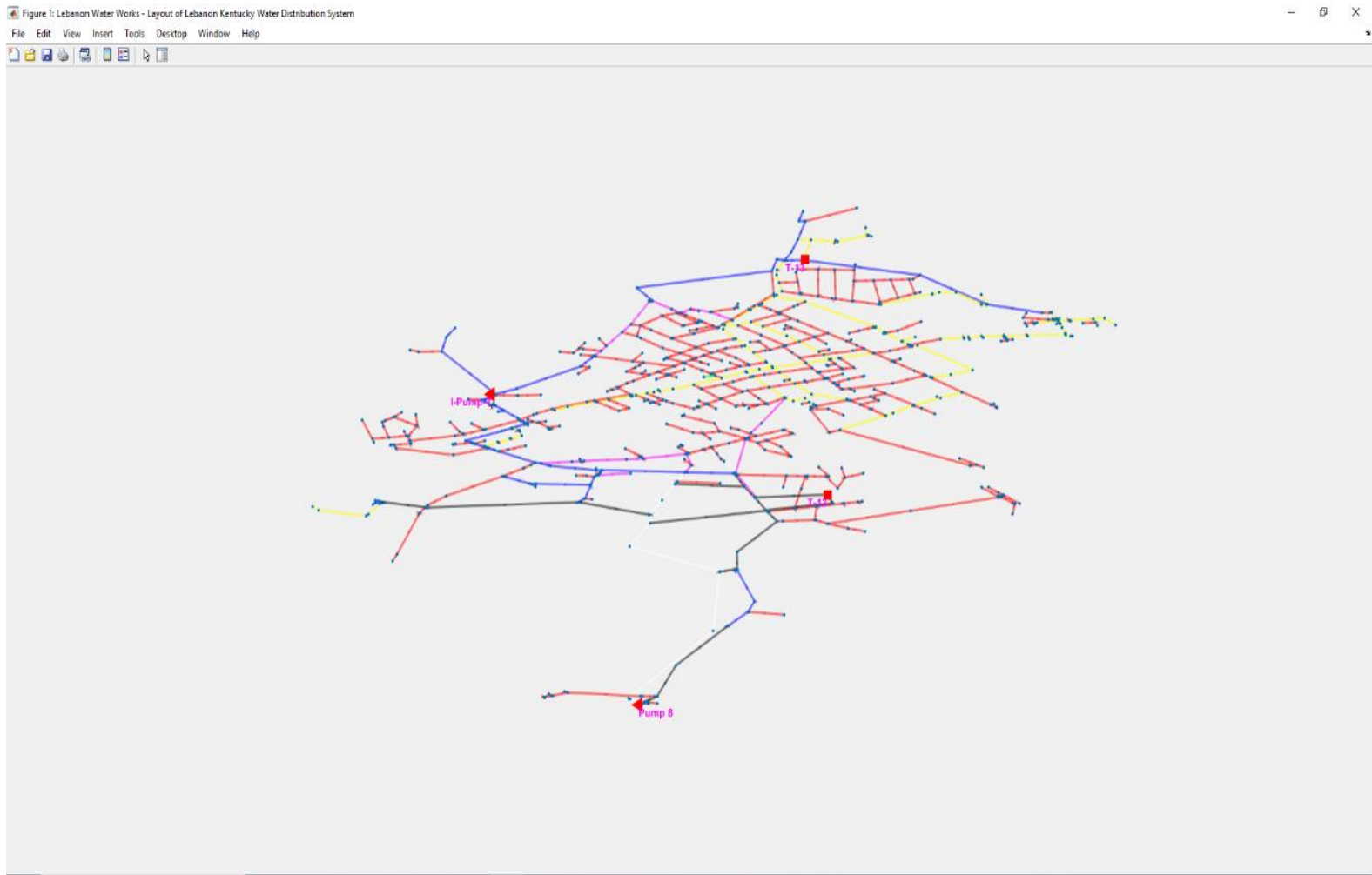
Figure 5-14: Generated Interactive Map of LWW Showing Pipe Diameters
