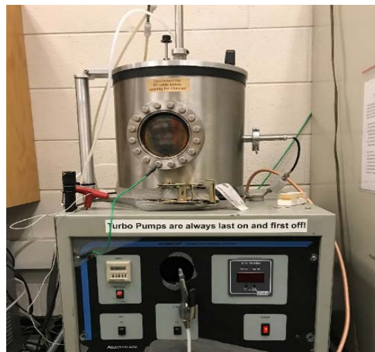
Figure 2.5 Sputtering deposition system.
