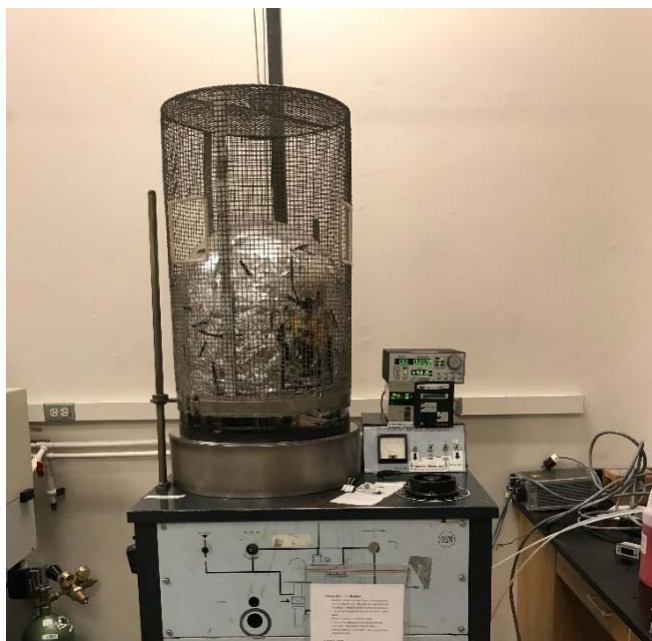
Figure 2.6 Thermal deposition system for gold electrode.
