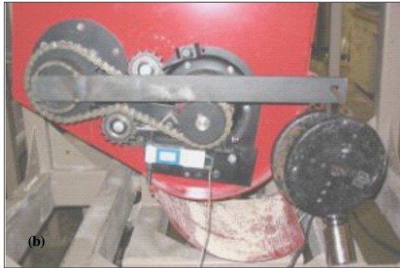
Figure 4. Static calibration apparatus. Lock arm (a) and moment arm (b).
