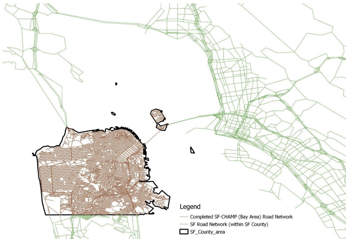
Figure 3-7: Clipping the SF County road network from the Bay Area road network
