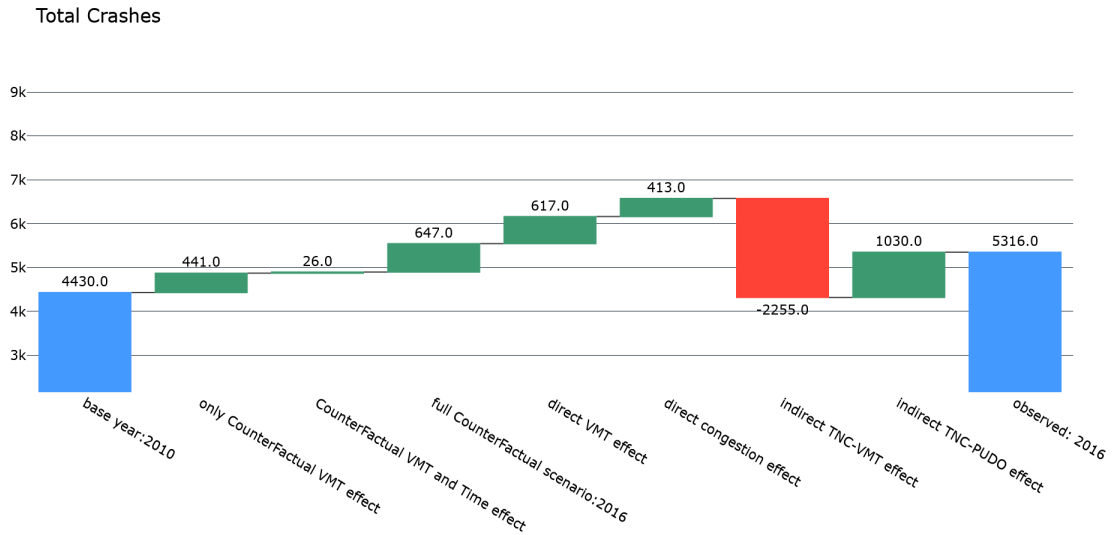
Figure 5-7: Scenario results for the dependent variable is equal to Total Crash (when Tot VMT is utilized as the exposure variable)
