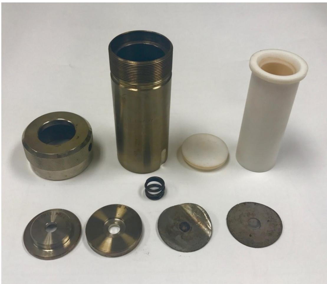
Figure 1.1 Disassembled parts of the hydrothermal reactor and the Teflon liner.
