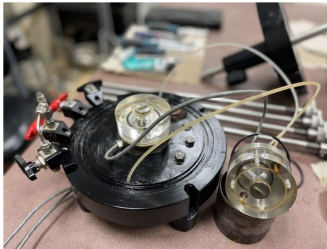
Figure 3-2 Top cap and pedestal of the testing equipment and the attached bender elements
