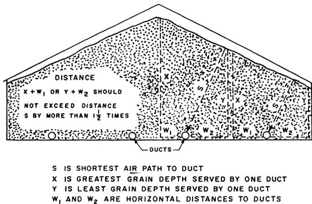
Fig. 2—Spacing configuration for lengthwise ducts in a peak loaded flat storage.
