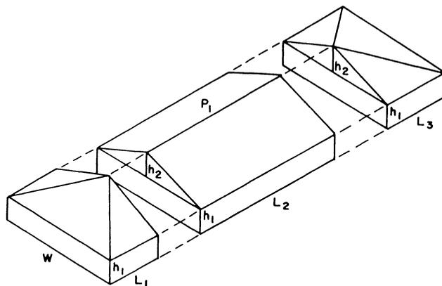
Fig. 1—The geometric volumes used to represent a peaked grain mass in a rectangular storage (Brook, 1983).
