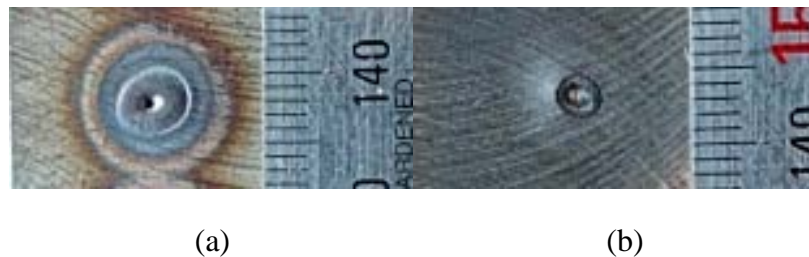
Figure 8-11 Surface appearance of the finished workpiece using stationary welding and MPC feedback control.
