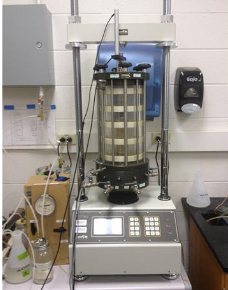
Figure E.3 Load frame and double walled unsaturated triaxial cell
