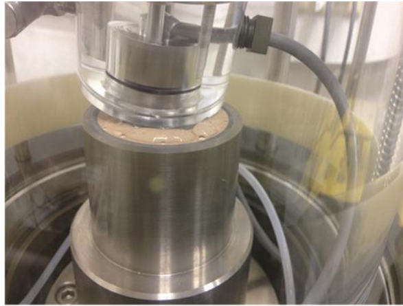
Figure E.10 Water pond formed on the surface of HAEPD through bottom-up process
