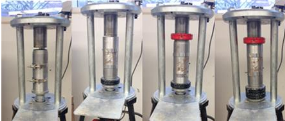
Figure E.8 Process of fabricating a compacted specimen for unsaturated Bender Element testing
