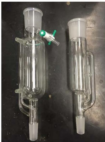
**Figure 3.8:** The specially-design Soxhlet extractor with water-jacket (left) and traditional Soxhlet extractor (right).
