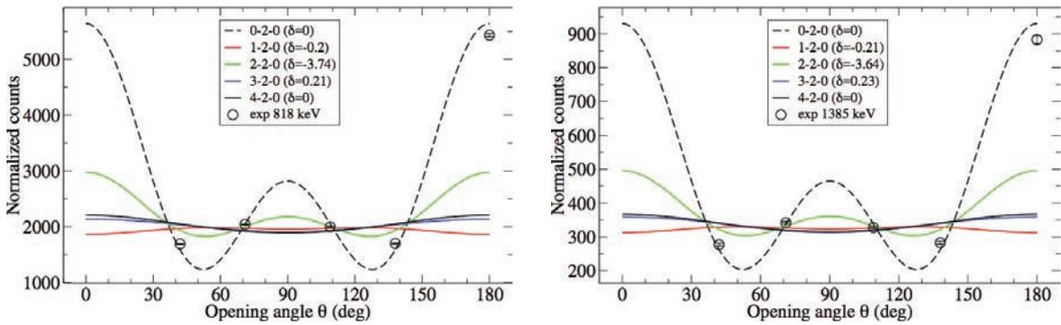
Fig. 2. Angular correlation of 818- and 331-keV  $\gamma$ -rays (left), 1385- and 331-keV  $\gamma$ -rays (right). Experimentally measured angular correlation counts normalized to the number of detector pairs and corrected for detector geometry effects are indicated in circle, while theoretically drawn curves for different possible cascades are given in different colours.
