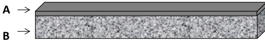
Figure 1.2: Schematic representation of an asymmetric flat sheet membrane. (A) \sim 0.1\text{-}1\ \mu\text{m} thick dense layer, where gas separation occurs via solution diffusion (B) \sim 100\text{-}200\ \mu\text{m} thick porous layer, which provides mechanical support.
