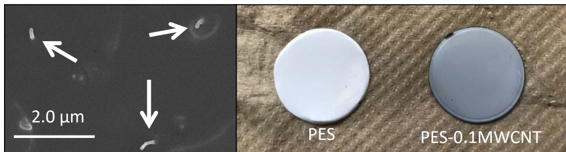
Figure 3.13: (Left) SEM image of PES-0.1MWCNT dense film cross-section. Arrows indicate MWCNTs. (Right) photograph of PES and PES-0.1MWCNT membrane coupons, showing macroscopic color change that accompanies MWCNT dispersion.
