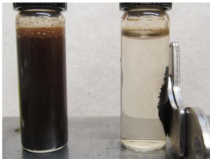
Figure 4.7 Dispersed ABDTH 2 MNPs and magnetically separated ABDTH 2 MNPs using computer hard drive magnets
