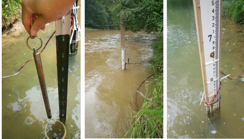
Figure 3.7 Image to far right is Xylem YSI InSitu® datalogger and still well at site 2. Middle and far right image is of stage-gage at site 2. Pictures taken by C. Peterman, dates vary.
