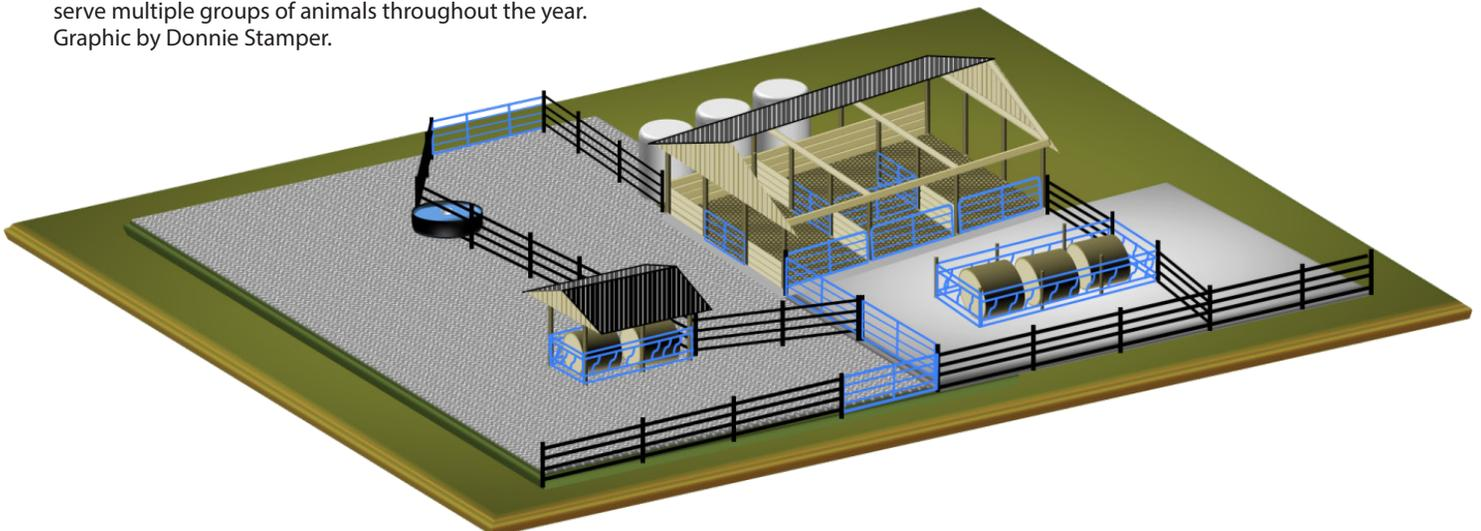
**Figure 2.** The bull barn consists of handling facilities, with a growing facility and maternity area. The complex utilizes water harvesting, runoff control, creep feeding, and winter-feeding areas. Solar power is used to provide water to two watering systems that serve multiple areas. The complex is designed to be used throughout the year. Graphic by Donnie Stamper.
