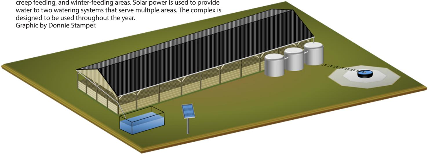
**Winter and drought feeding area:** All-weather surfaces including concrete, geotextile fabric, and rock are used for controlling mud, limiting erosion, minimizing maintenance diets, and reducing mortalities.
