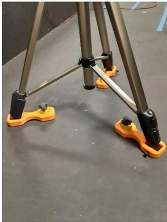
Figure 4.3 Camera Tripod with Magnets
