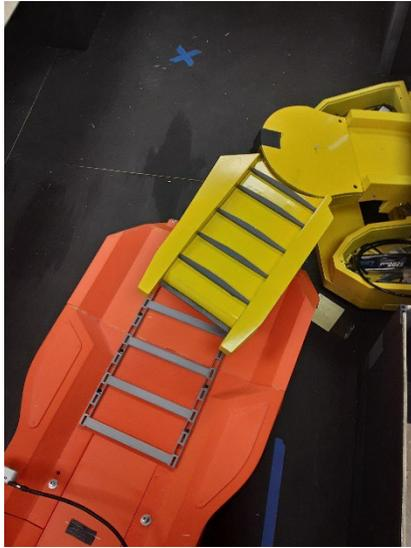
Figure 6.10 Shuttle Car Docked Correctly Under Miner Conveyor
