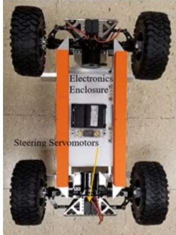
Figure 3.3 One-Sixth Scale Shuttle Car Chassis
