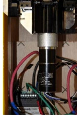
Figure 3.4 Traction Motor Mounted to Axle Gearbox
