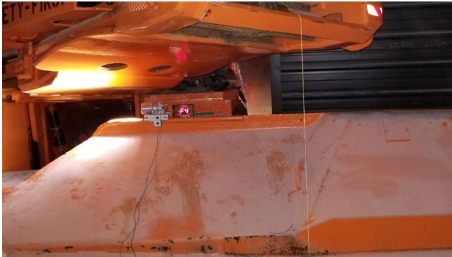
Figure 5.10 Externally Mounted Headlight to Shuttle Car Load-End
