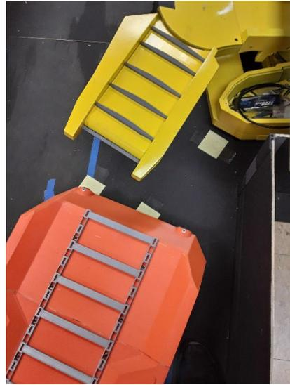
Figure 6.11 Shuttle Car Incorrectly Docked, Short of Conveyor
