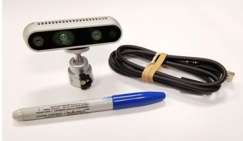
Figure 4.1 Intel's RealSense D435i Camera
