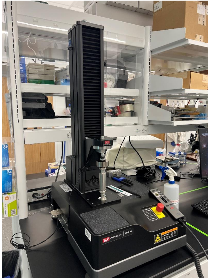
Figure 8: Instron used for Mechanical Testing
