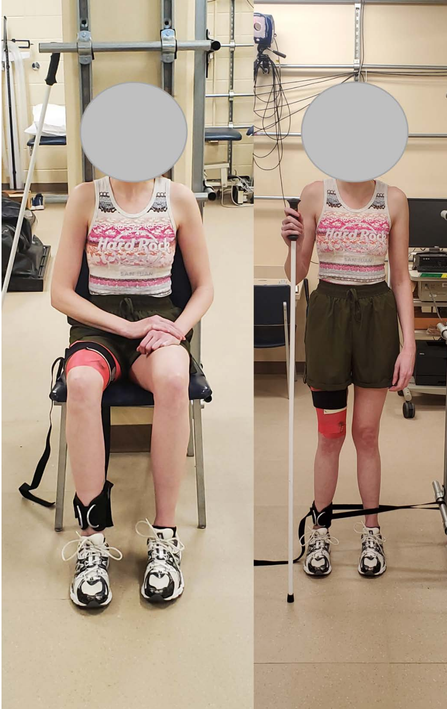
Figure 3.1: Testing procedure for collecting maximal voluntary isometric contractions (MVIC) for the quadriceps (left) and gluteus medius (right) musculature.
