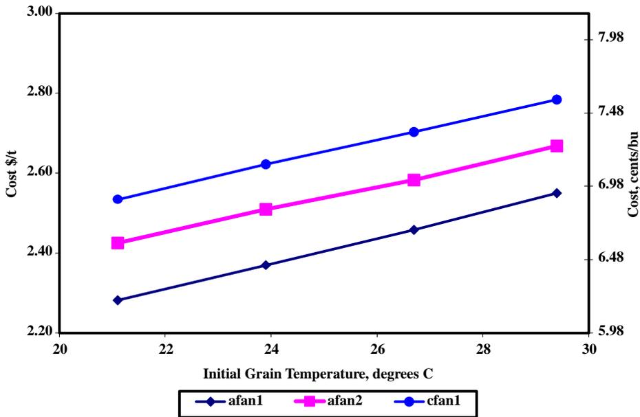
Figure 3. Average aeration costs in \$/t and cents/bu vs. initial grain temperature for the three fans in this study using 30 yrs of weather for Lexington, Kentucky, a 15 June harvest date and an aeration temperature window of 0 to 17°C.
