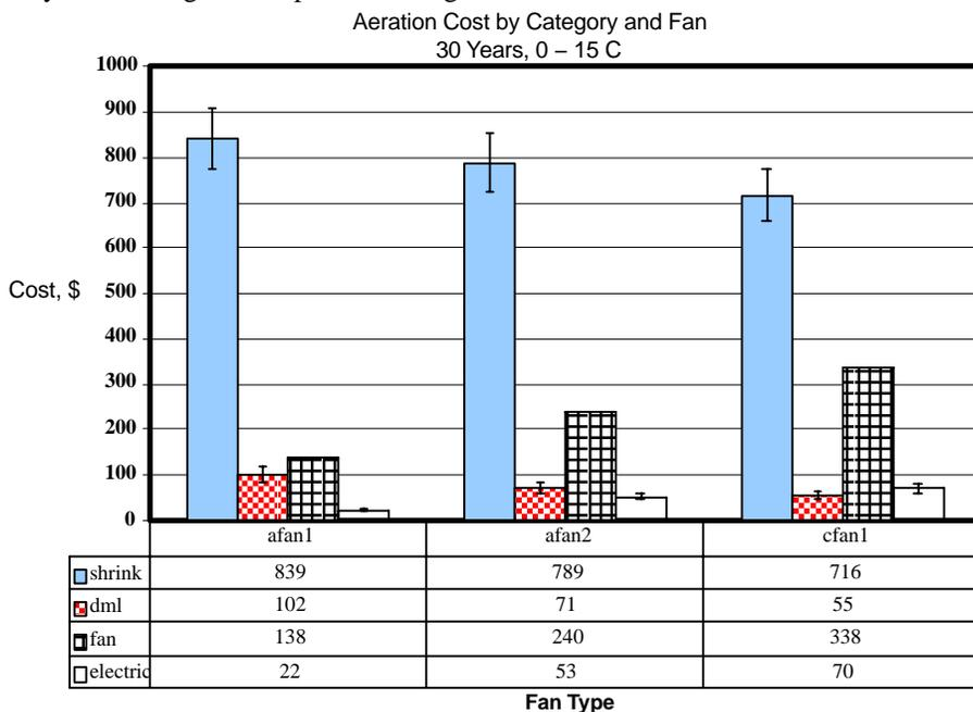
Figure 1. The 30-yr average values and standard deviation bars for the aeration cost components of shrinkage, dry matter loss, owning the fan and electricity use by fan type for Lexington, Kentucky, weather data, four starting dates, four initial grain temperatures and a 0 to 15°C temperature window.
