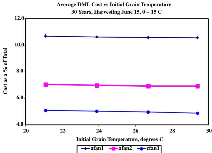
Figure 8. The average cost of the dry matter loss (DML) of wheat as a percent of the total aeration cost for the three fans in this study using 30 yrs of weather for Lexington, Kentucky, a 15 June harvest date and an aeration temperature window of 0 to 15°C.
