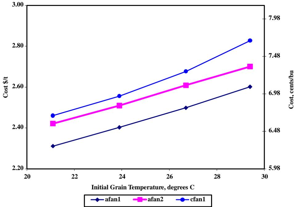
Figure 2. Average aeration costs in \$/t and cents/bu vs. initial grain temperature for the three fans in this study using 30 yrs of weather for Lexington, Kentucky, a 15 June harvest date and an aeration temperature window of 0 to 15°C.
