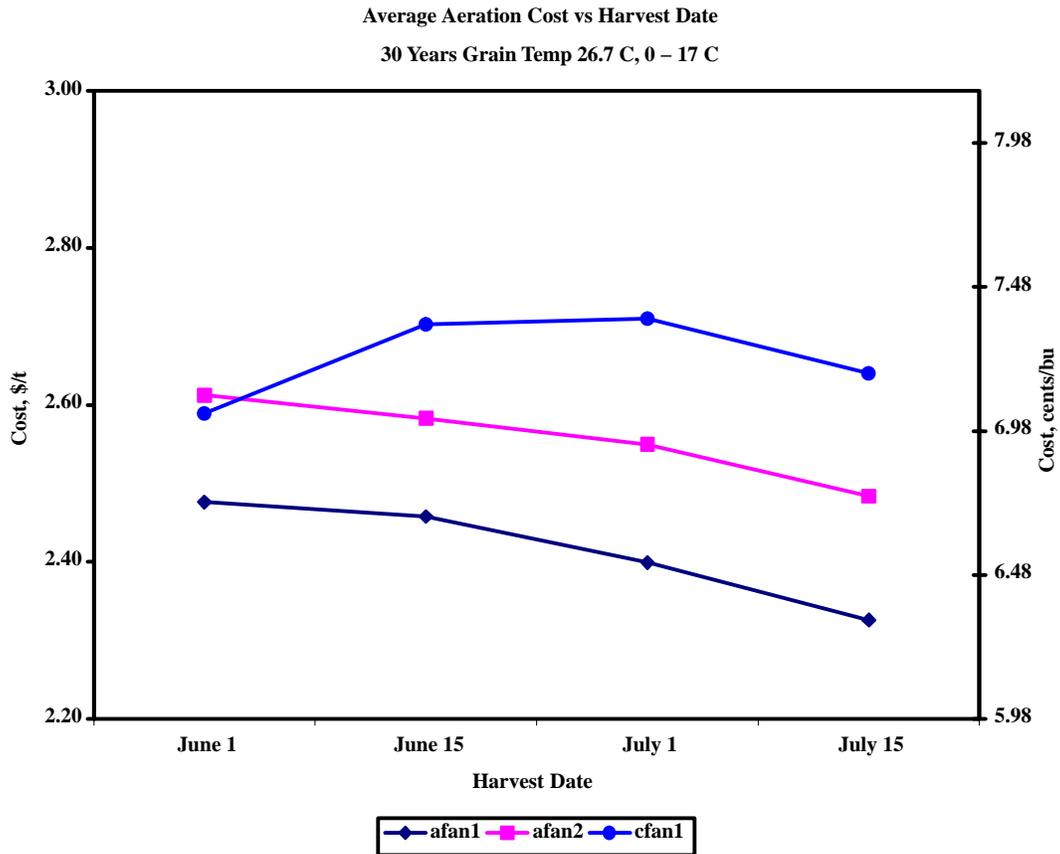
Figure 5. Average aeration costs in \$/t and cents/bu vs. harvest date for the three fans in this study using 30 yrs of weather for Lexington, Kentucky, an initial grain temperature of 26.7°C (80.0°F) and an aeration temperature window of 0 to 17°C.
