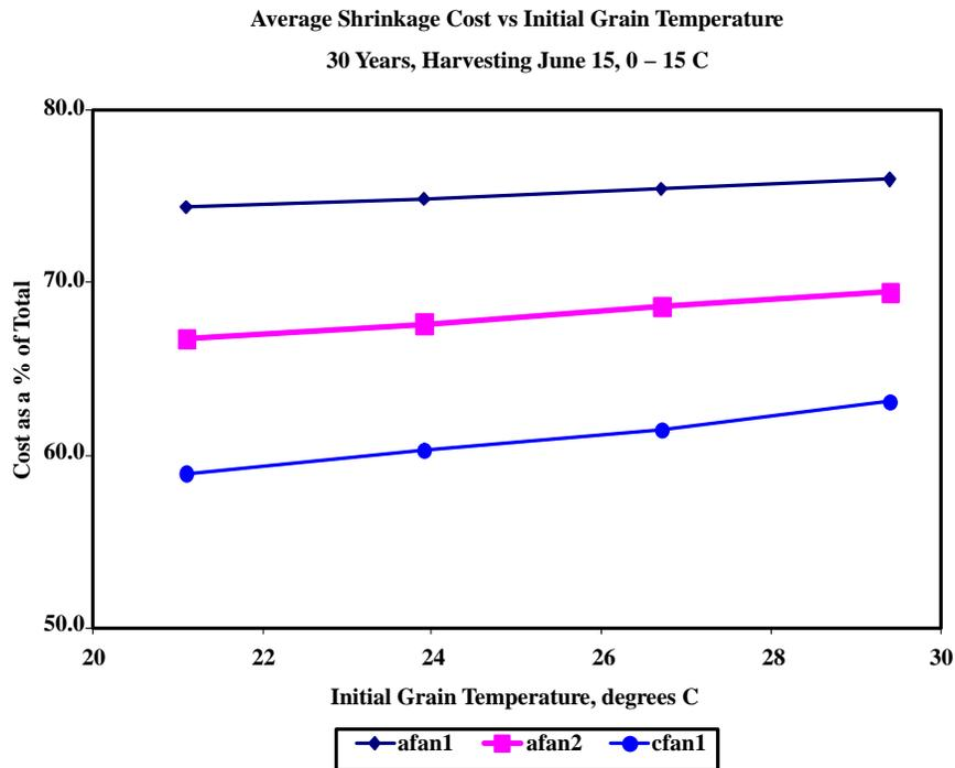
Figure 6. The average cost of the wheat shrinkage as a percent of the total aeration cost for the three fans in this study using 30 yrs of weather for Lexington, Kentucky, a 15 June harvest date and an aeration temperature window of 0 to 15°C.
