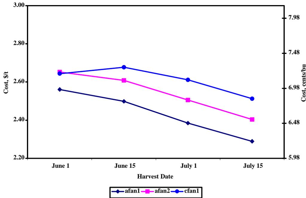
Figure 4. Average aeration costs in \$/t and cents/bu vs. harvest date for the three fans in this study using 30 yrs of weather for Lexington, Kentucky, an initial grain temperature of 26.7°C (80.0°F) and an aeration temperature window of 0 to 15°C.
