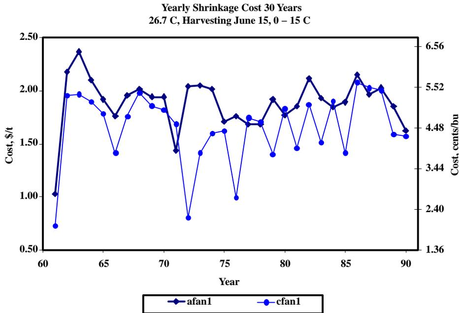
Figure 7. The yearly shrinkage cost (\$/t) of wheat due to aeration for the fans afan1 and cfan1 in this study using 30 yrs of Lexington, Kentucky weather beginning harvest on 15 June, with an initial grain temperature of 26.7°C (80°F) and an aeration window of 0 to 15°C.
