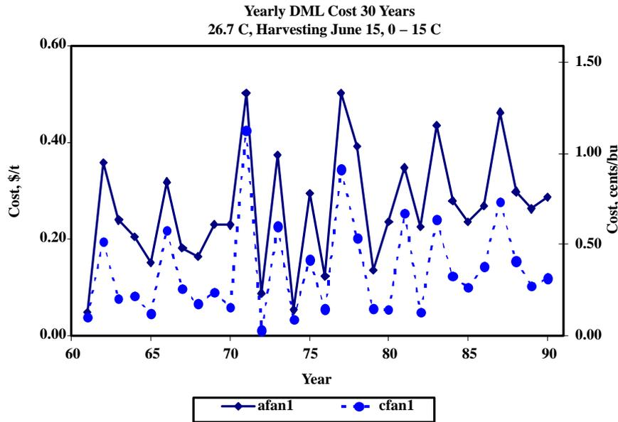
Figure 9. The yearly cost (\$/t) of dry matter loss (DML) due to aeration for the fans afan1 and cfan1 in this study for 30 yrs of Lexington, Kentucky weather beginning harvest on 15 June, with an initial grain temperature of 26.7° C (80° F) and an aeration window of 0 to 15° C.
