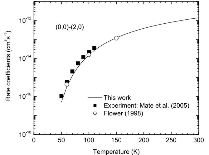
FIG. 1.—Rate coefficients for  $(0, 0) \rightarrow (2, 0)$  rotational excitation in indistinguishable H<sub>2</sub>+H<sub>2</sub> collisions as a function of temperature. The solid curve denotes the present result, which uses the Diep & Johnson (2000) PES. The filled squares represent the experimental data from Maté et al. (2005). The open circles represent the theoretical results of Flower (1998).
