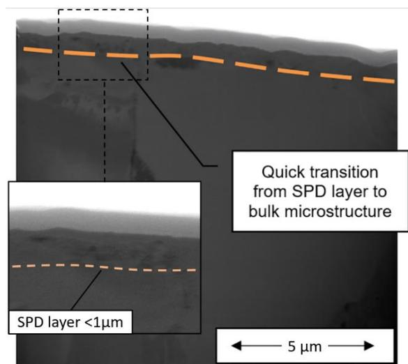
Fig. 9. FIB micrograph of near-surface microstructure of sample machined with 5 $\mu\text{m}$  hone edge, 0.4mm tool nose radius and 0.1mm feed. FIB microscopy, 8000x.
