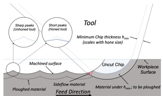
Fig. 3. Geometrical model of a turning process clarifying the influence of ploughing effects on roughness at higher kinematic roughness values. Note that  $h_{min}$  is meant to denote minimum chip thickness.
