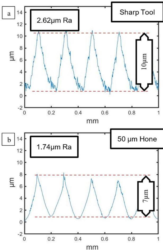
Fig. 7. Laser interferometer-generated surface cross sections showing the relative differences of roughness profiles at higher kinematic roughness. a) 0.8mm nose radius, 0.2mm feed, 5 $\mu\text{m}$  hone. b) 0.8mm nose radius, 0.2mm feed, 50 $\mu\text{m}$  hone.
