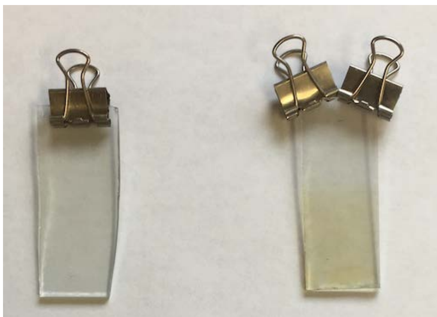
Figure 8.3. An untreated TiO 2 film (left) compared to a dopamine treated TiO 2 film (right).
