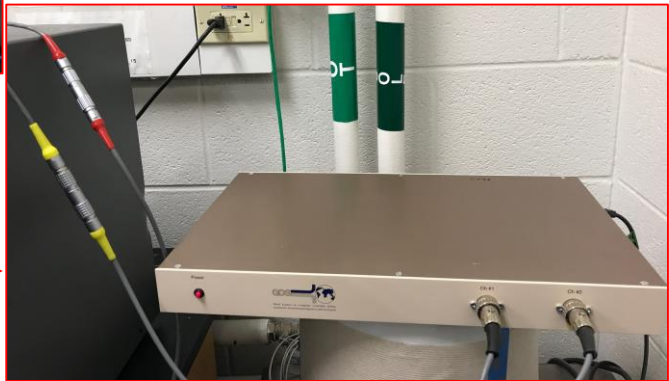
Figure D-6 connecting triaxial cell and signal processor that analyzes the generated waves.
