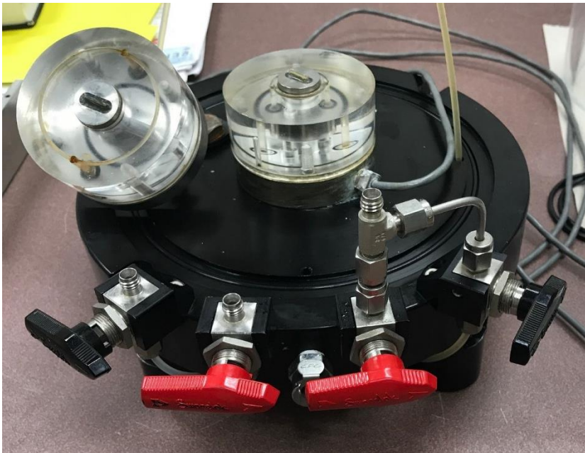
Figure D-3 the two bender elements mounted in the top and bottom caps of the triaxial cell.
