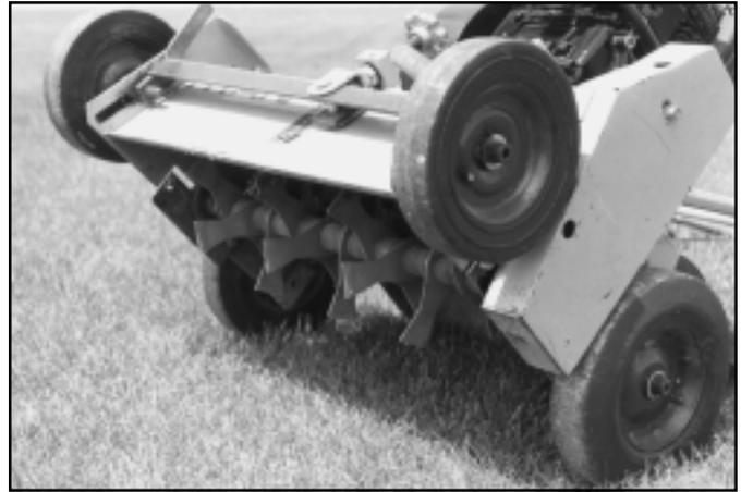
*A good thatching machine has fixed knives or sling blades; spring tines are not effective.*
