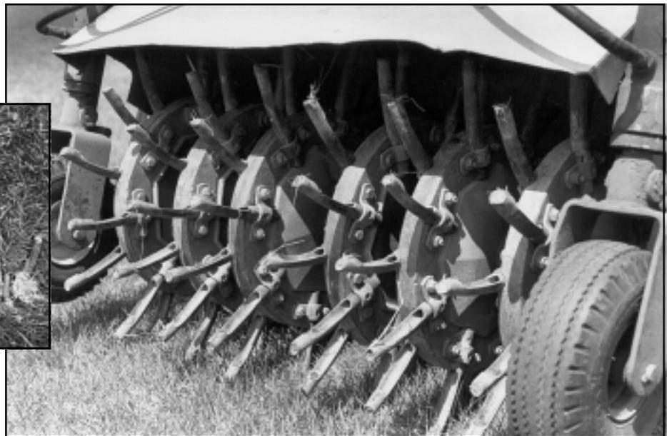
*Coring machines remove plugs of soil and grass and open up the soil for improved aeration and water infiltration.*
