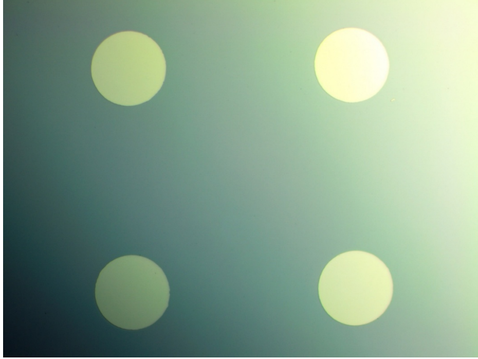
Figure 2.5. Ni gate of MOS capacitors fabricated using wet etching process.
