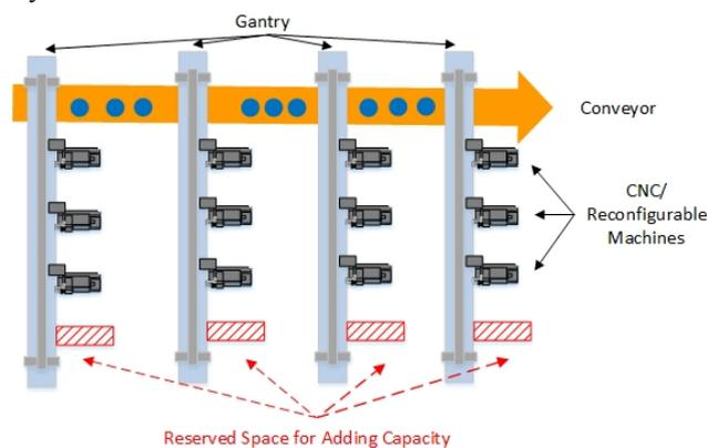
**Figure 2:** A typical RMS architecture
