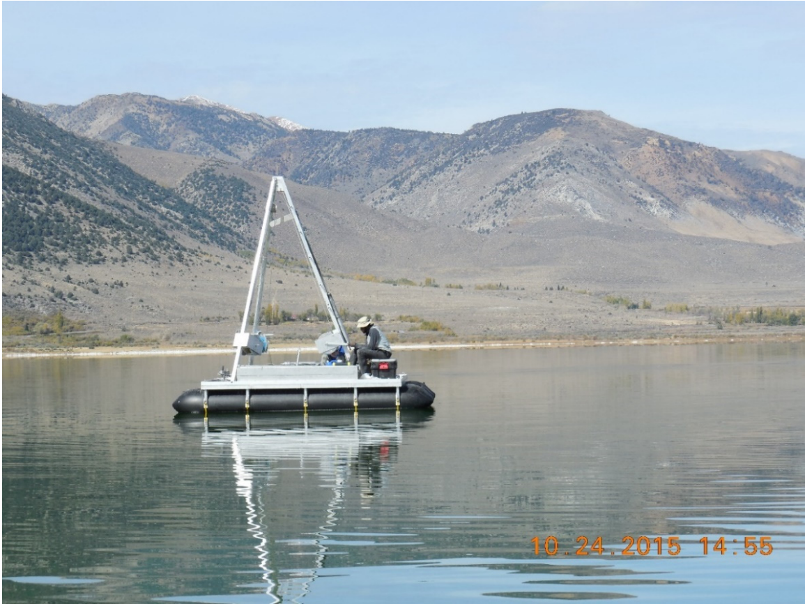
Figure 5: Photo of the UK-UWITEC percussion piston coring barge deployed on Mono Lake. Using this system, we were able to core through tephras and preserve delicate sedimentary structures.
