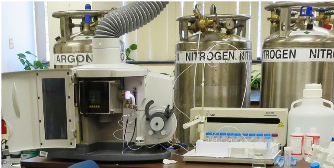
Figure 3.17. ICP-OES apparatus at Kentucky Geological Survey at used for elemental characterization of the aqueous phase.
