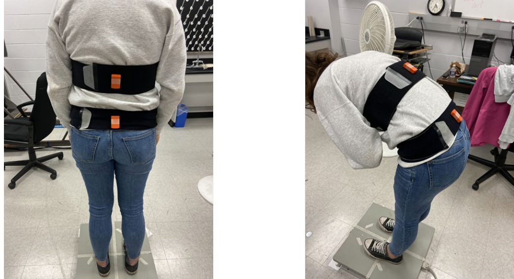
Figure 2.1: IMU placement over T10 and S1 vertebrae while standing and during forward bending task
