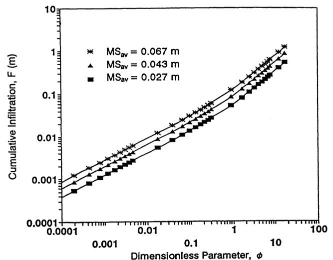
Figure 2—Cumulative infiltration ( $F$ ) vs.  $\phi$  for three values of  $MS_{av}$ . Solid lines represent the predicted value from equation 3 and the symbols represent actual values from the modified Green-Ampt equation (eq. 1).
