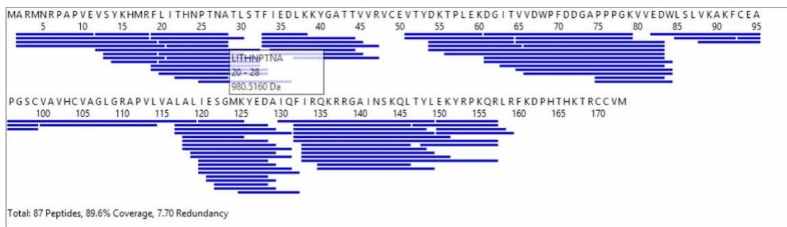
Figure 3.9. Sequence coverage map of apo-PRL-3 in HDX-MS. After mass spectrometry, all deuterated peptides were mapped back to the PRL-3 amino acid sequence. Each blue bar represents a detected peptide. The high coverage and redundancy of PRL-3 peptides indicated that epitope mapping experiments would yield high-quality data. 1 \mu l of 40 \mu M PRL-3 was used for deuterium exchange; the reaction was quenched with 200 \mu l 1XQ (0.5 mM Guanidine HCl); 100 \mu l was injected for mass spectrometry analysis. 87 peptides were detected with a redundancy score of 7.70. 89.6% of PRL-3 was mapped with these peptides.
