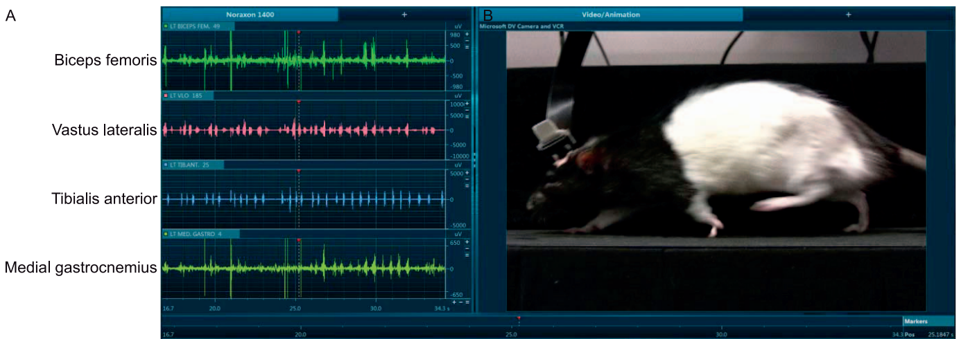
Figure 3. The in vivo collection of electromyography (EMG) during unconstrained walking on a motor-driven treadmill (16 m/min). A, The EMG signals of the left instrumented hind limb were synchronized with a high-speed camera. B, The rat and head connector were attached to the fine-wire EMG and the EMG data-acquisition system.
