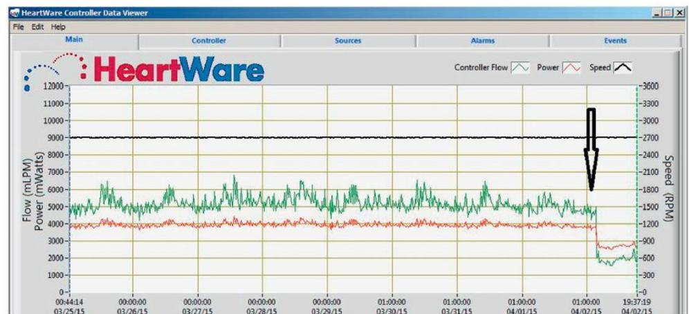
Screen shot of left ventricular assist device log-file analysis, pertaining to pump power and flow trends. The onset of low flow, caused by wedge thrombus occluding the inflow cannula, is acute within hours. **Arrow** indicates exactly the abrupt onset of low flow. Courtesy of HeartWare.
