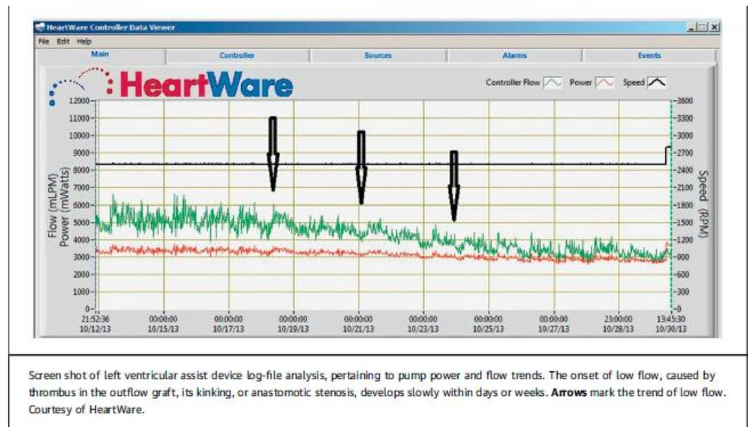
**Figure 5.** Gradual decrease of flow due to obstruction in the outflow graft. Reproduced from Scandroglio et al. (71), with permission.
