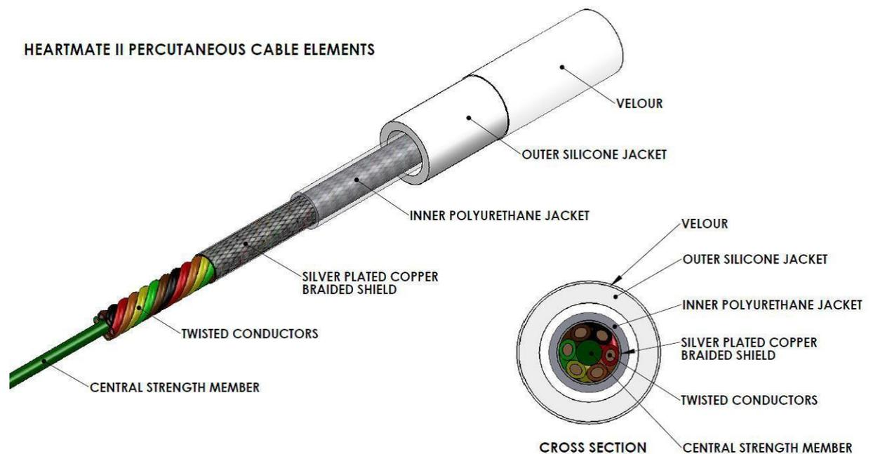
**Figure 1. Structure of the driveline** (reproduced with permission of Thoratec)
