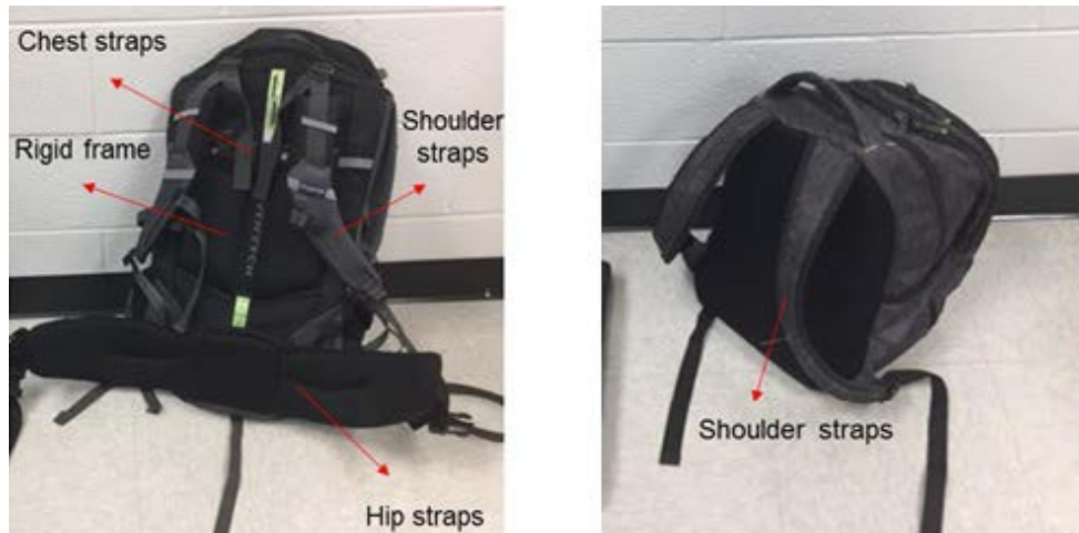
Figure 3-1 The ergonomically modified (left) and normal (right) backpacks used in this study. Each backpack was filled by letter size papers to generate a backpack weight equal to 10% of participant's body weight.
