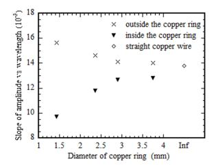
Figure 5.5 Variation of the slope of the amplitude to the wavelength with the size of the copper ring (film thickness: 90 nm)
