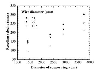
Figure 8.6 Variation of the average receding velocity of the contact line with the diameter of copper ring for three wire diameters (film thickness: ~90 nm)
