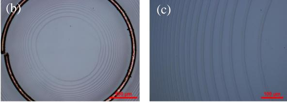
Figure 8.1 (a) Schematic of the cross section of a toluene droplet confined by a copper ring on a PMMA film; (b-c) Optical images of the evaporation–induced gradient concentric rings on a pre-cast PMMA film (film thickness: ~140 nm; diameter of the copper ring: 2560  $\mu$ m); (b) a large view of the surface pattern, and (c) an enlarged view of the pattern inside the copper ring.
