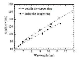
Figure 5.4 Correlation between the amplitude and the wavelength of the concentric rings formed via a copper ring of 2360  $\mu$ m in diameter (film thickness: 140 nm)
