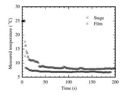
Figure 7.2 Temporal evolution of the temperature of the cooling stage and the surface temperature of a pre-cast PMMA film of  $\sim$ 140 nm thickness
