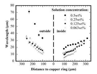
Figure 5.12 Variation of wavelength with the distance to copper ring for four solution concentrations (copper ring diameter: 1380  $\mu$ m, substrate temperature: 21 °C)
