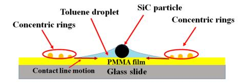
Figure 3.1 Schematic of the evaporation of a toluene droplet via a "particle-on-film" template and the formation of gradient concentric PMMA rings on a pre-cast PMMA film
