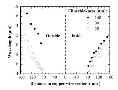
Figure 5.6 Variation of the wavelength with the distance to copper ring (diameter of copper ring: 1425  $\mu$ m). "0" in the x-axis refers to the position of the copper wire.
