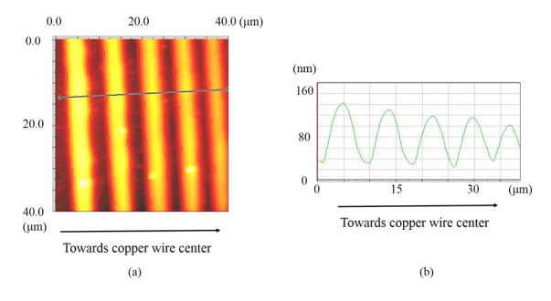
Figure 4.2 (a) An AFM image of the parallel stripes over an area of  $40 \times 40 \ \mu m^2$ , and (b) surface profile of the parallel stripes (film thickness: 90 nm; copper wire diameter 79  $\mu m$ )
