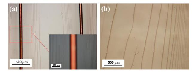
Figure 4.6 (a) Optical images of the evaporation–induced surface patterns formed *via* two parallel copper wires (Inset: enlarged view of the pattern in the rectangular box), and (b) surface patterns far away from the copper wires (film thickness: 90 nm; diameter of the copper wire: 79 mm)
