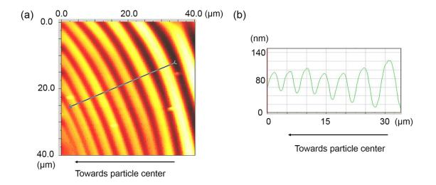
Figure 3.3 (a) AFM image of the concentric rings over an area of  $40 \times 40 \ \mu\text{m2}$ , and (b) surface profile of the concentric rings (film thickness: 135 nm; average particle diameter:  $160 \pm 29 \mu\text{m}$ )
