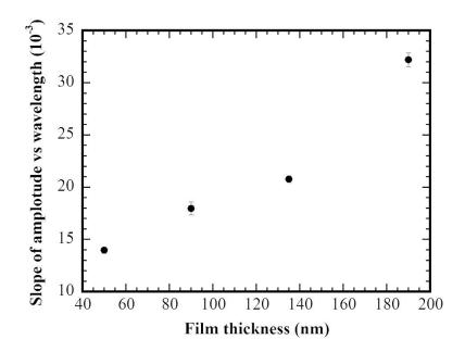
Figure 3.9 Dependence of the slope of the amplitude verse the wavelength on film thickness (average particle diameter:  $160 \pm 29 \mu m$ )
