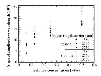
Figure 5.13 Variation of the slope of the amplitude to the wavelength with the solution concentration (substrate temperature: 21  $^{\circ}$ C)
