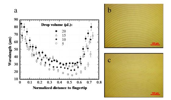
Figure 6.3(a) Variation of the wavelength with the normalized distance to the finger tip for different droplet volumes(tilt angle: 2.86°, film thickness: ca. 90nm);(b and c) Optical images of the typical multiple arc-ridges formed along the symmetric axis for different droplet volumes of  $10\mu$ L (b) and  $5\mu$ L (c)(tilt angle: 2.86°, normalized distance:0.5, film thickness: ca. 90nm)
