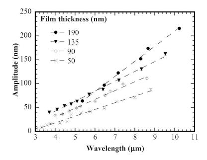
Figure 3.8 Correlation between the wavelength and the amplitude of smooth concentric rings for four film thicknesses (average particle diameter:  $160 \pm 29 \mu m$ )
