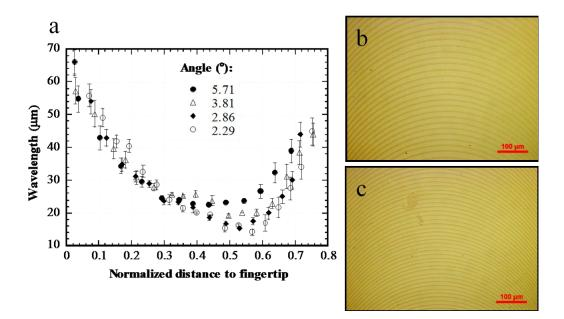
Figure 6.4 (a) Variation of the wavelength with normalized distance for four different tilt angles(droplet volume:  $5\mu$ L, film thickness: ca. 90 nm); (b) and (c) optical images of the multiple arc-ridges formed along the symmetric axis for two tilt angles of 5.71° (b) and 2.29° (c) (droplet volume:  $5\mu$ L,normalized distance:0.5)
