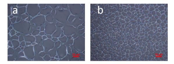
Figure 7.9 Surface patterns formed on a PS film via the evaporation of a toluene droplet: (a) in zone 1, and (b) in zone 2 (film thickness:  $\sim$ 290 nm, equilibrium temperature of the film surface:  $\sim$ 8.0 °C, diameter of the copper ring: 1.45 mm)
