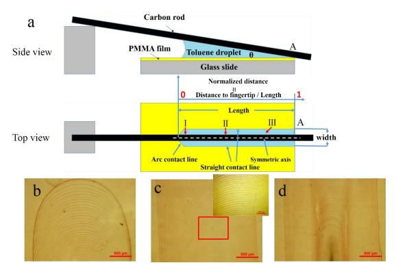
Figure 6.1(a) Schematic of the experimental set-up for constructing finger-like surface patterns, and (b-d) the surface patterns formed in the regions of I, II and III indicated in (a). The inset in (c) is an enlarged view of the patterns enclosed in the red box (film thickness: ca. 90 nm; tilt angle:  $2.86^{\circ}$ ; droplet volume:  $5\mu$ L)
