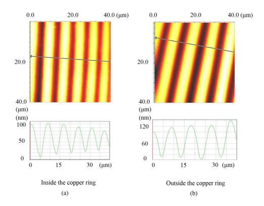
Figure 5.2 AFM images and line scans of the concentric rings nearest to a copper ring over an area of  $40 \times 40 \ \mu m^2$  (film thickness: 140 nm; diameter of the copper ring: 2360  $\ \mu m$ ); (a) the PMMA rings inside the copper ring, and (b) the PMMA rings outside the copper ring
