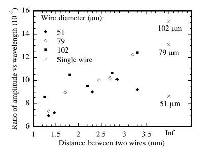
Figure 4.8 Variation of the slope of amplitude verse wavelength with the distance between two copper wires for three copper wires (film thickness: 90 nm)
