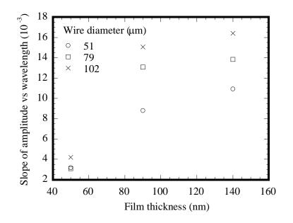
Figure 4.5 Variation of the slope of amplitude verse wavelength of smooth stripes (formed *via* a single copper wire) with film thickness for three wire diameters
