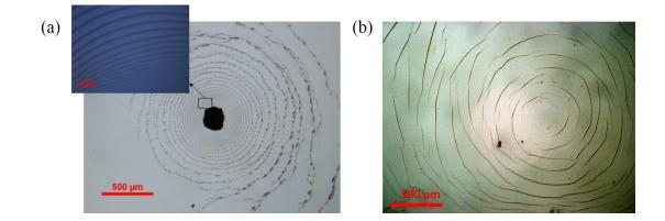
Figure 3.2 Optical images of the evaporation–induced surface patterns: (a) surface pattern with a particle in the drop (film thickness: 135 nm; average particle diameter:  $160 \pm 29 \mu m$ ), and (b) surface pattern without a particle in the drop (film thickness: 135 nm)
