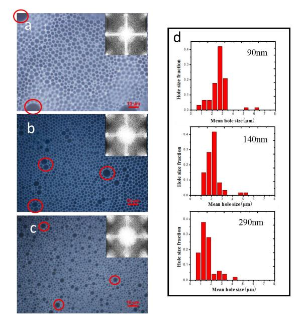
Figure 7.3 Surface patterns formed in zone 1 on different PMMA films; (a) ~90 nm in thickness, (b) ~140 nm in thickness and (c) ~290 nm in thickness; (d) size distribution of the holes formed on the PMMA films (surface temperature of the PMMA at equilibrium: ~8 °C, the diameter of the copper ring is 1.45 mm). Inserted images are the Fast Fourier Transform (FFT) patterns of the corresponding surface patterns.
