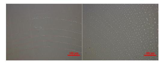
Figure 6.6 Optical images of the typical surface patterns formed on polystyrene (PS) film (tilt angle: 2.86°, film thickness: ca. 90nm). (a) along the symmetric, normalized distance: 0.25; (b) the transition zone of the arc-segment and the straight line-segment, normalized distance: 0.25.
