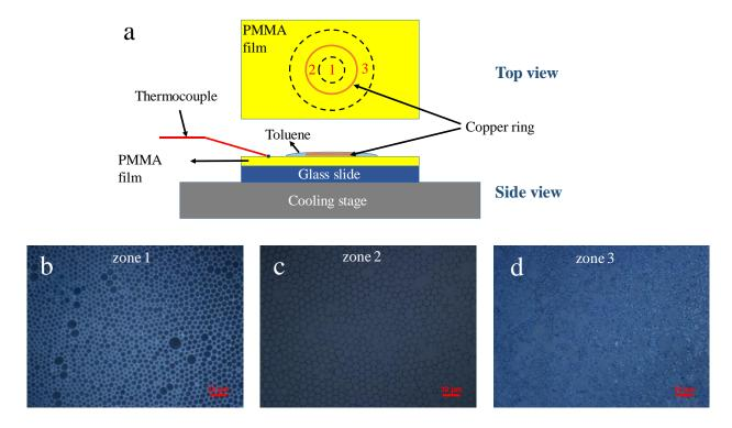
Figure 7.1 (a) Schematic of the experimental setup; (b-d) surface patterns formed in the zones of 1-3 as labeled in Fig. 1a, respectively (film thickness: ~140 nm, the diameter of the copper ring is 1.45 mm, surface temperature of the film at equilibrium: 8 °C)
