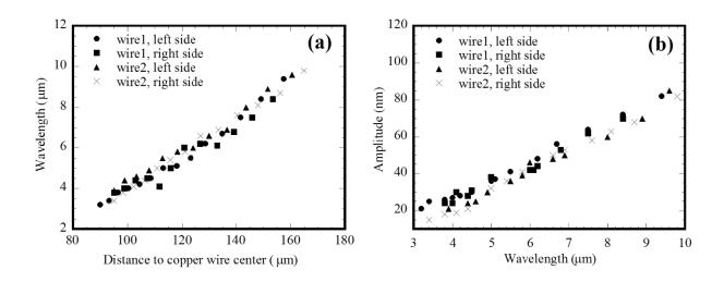
Figure 4.7 (a) Variation of the wavelength of smooth stripes with the distance to individual copper wire centers, and (b) correlation of the amplitude and the wavelength of the smooth stripes formed *via* two copper wires (diameter of the copper wires: 79  $\mu$ m; distance between two copper wire centers: 1.7 mm; film thickness: 90 nm)
