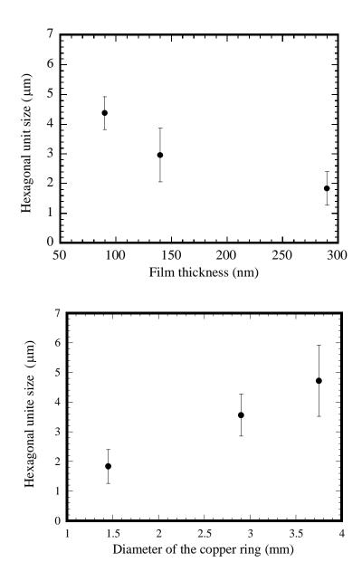
Figure 7.11 (a) Size variation of the hexagonal unit with the PMMA film thickness, and (b) size variation of the hexagonal unit with the copper ring diameter (film thickness: 290 nm, surface temperature of the film at equilibrium state:  $\sim$ 8.0 °C).
