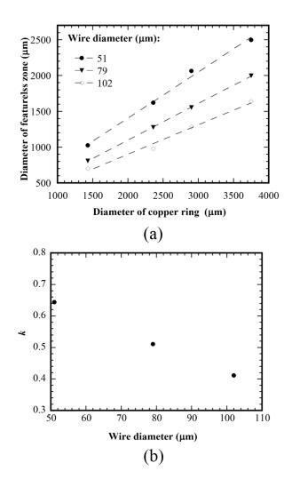
Figure 8.3(a) Variation of the size of the featureless zone with the diameter of the copper rings of three wire diameters for the patterns formed on the PMMA films of  $\sim$ 90 nm thickness, and (b) variation of the slope of the linear fitting of the results in (a) with the wire diameter.
