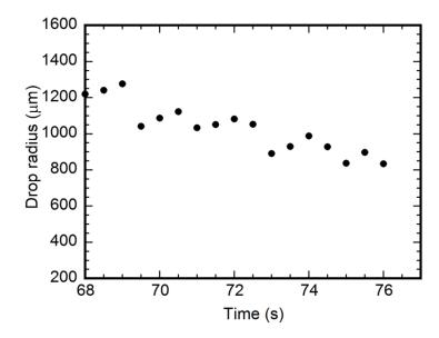
Figure 3.10 Variation of the drop radius with evaporation time during a toluene drop evaporating on a PMMA film with a particle in the drop (film thickness: 135 nm; average particle diameter:  $160 \pm 29 \mu$ m).
