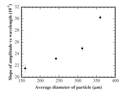
Figure 3.6 Dependence of the slope of the amplitude verse the wavelength on the particle size (film thickness: 135 nm)
