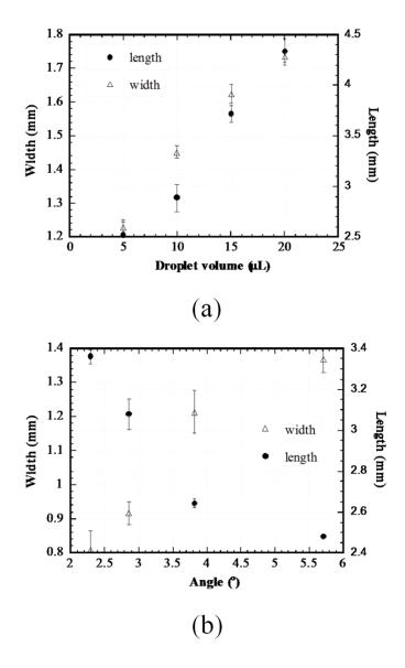
Figure 6.2 (a) Variation of the dimensions of the outmost finger-like pattern with the droplet volume (tilt angle:  $2.86^{\circ}$ , film thickness: ca. 90nm); (b) Variation of the dimensions of the outmost finger-like pattern with tilt angle (droplet volume:  $5\mu$ L, film thickness: ca. 90nm).
