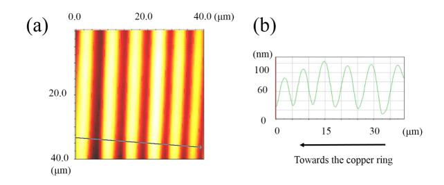
Figure 8.2(a) AFM image of the concentric rings over an area of  $40 \times 40 \ \mu m^2$ , and (b) surface profile of the concentric rings. (film thickness: ~90 nm; diameter of the copper ring: 2560  $\mu m$ )
