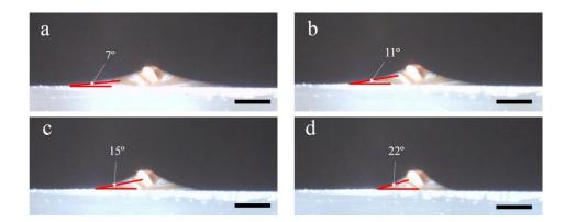
Figure 8.8 Side-view of the digital images of a toluene droplet confined by a straight copper wire of 25 mm in length and 500  $\mu$ m in diameter. The distance from the contact line to the copper wire: (a) 1875  $\mu$ m; (b) 1450  $\mu$ m; (c) 1180  $\mu$ m and (d) 715  $\mu$ m. The nominal contact angle is noted by red line. The scale bars in all the images represent 1 mm.
