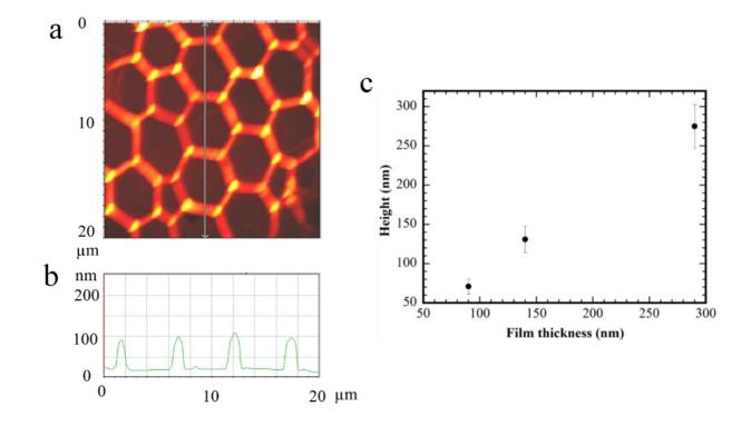
Figure 7.8 (a) A typical AFM image of the hexagon network formed in zone 2 on a PMMA film of ~90 nm thickness, (b) a line scan of the surface profile corresponding to the line in (a), and (c) variation of the wall height of the hexagon network with the film thickness (surface temperature of the film at equilibrium state: ~8.0 °C)
