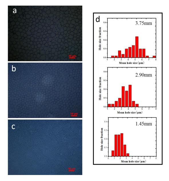
Figure 7.6 Surface patterns formed in zone 1 on PMMA films with copper rings of different sizes (a)  $\sim$ 3.75 mm in diameter, (b)  $\sim$ 2.90 mm in diameter, and (c)  $\sim$ 1.45 mm in diameter; (d) size distribution of the holes formed on the PMMA films (film thickness: 290 nm, surface temperature of the films at equilibrium:  $\sim$ 8 °C)
