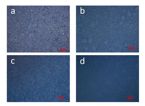
Figure 7.7 Surface patterns formed in zone 2 on the PMMA films of ~290 nm film thickness at four equilibrium temperatures; (a) -3.5 °C, (b) ~1.8 °C, (c) ~6.0 °C and (d) ~8.0 °C (copper ring size: 1.45 mm).
