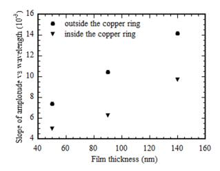
Figure 5.7 Dependence of the slope of the amplitude to the wavelength of the gradient concentric rings on film thickness (diameter of copper ring:  $1425 \mu m$ )
