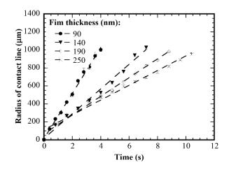
Figure 8.9 Variation of the radius of the internal contact line with time for four film thicknesses (diameter of copper wire: 79  $\mu$ m; diameter of copper ring: 3750  $\mu$ m). The time for the onset of the internal contact line is referred to as the reference time (0s).
