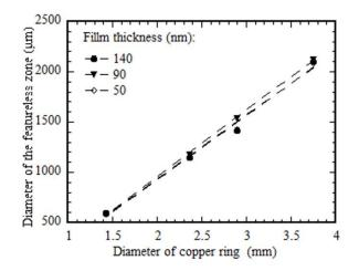
Figure 5.8 Variation of the size of featureless zone with the diameter of copper ring for three film thicknesses
