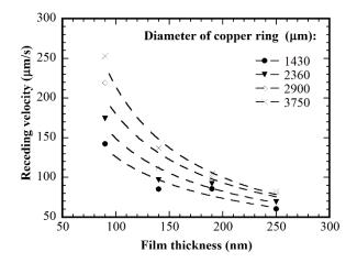
Figure 8.10 Variation of the average receding velocity of the contact line with film thickness for four ring diameters (wire diameter:  $79 \mu m$ )
