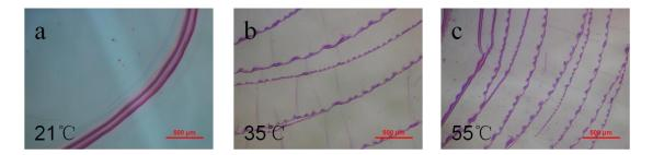
Figure 5.19 Optical images of the patterns formed by evaporating a droplet of PMMA solution in toluene on a glass slide without templates at different substrate temperatures: (a)  $21^{\circ}$ C, (b)  $35^{\circ}$ C and (C)  $55^{\circ}$ C. Solution concentration is 0.125wt%.
