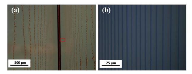
Figure 4.1 Optical images of the evaporation–induced surface patterns; (a) surface pattern formed *vis* a single copper wire, and (b) enlarged view of the surface pattern in the enclosed area in (a) (film thickness: 90 nm; diameter of the copper wire:  $79 \mu m$ )
