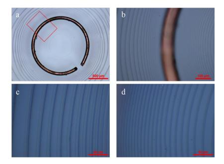
Figure 5.1 Optical images of the evaporation–induced gradient concentric rings on a precast PMMA film (film thickness: 140 nm; diameter of the copper ring: 1425  $\mu$ m); (a) a large view of the surface pattern, (b) an enlarged view of the surface pattern in the enclosed area in (a), (c) the concentric rings outside the copper ring, and (d) the concentric rings inside the copper ring
