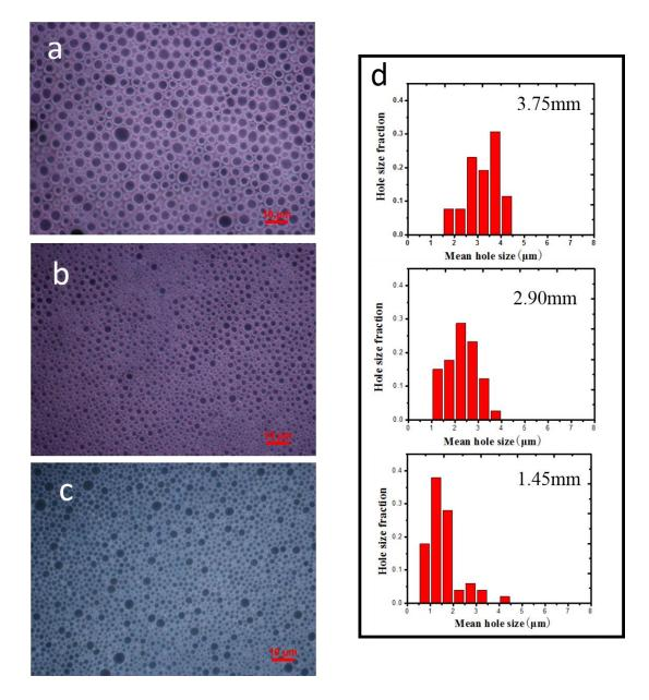
Figure 7.5 Surface patterns formed in zone 1 on PMMA films with copper rings of different sizes (a)  $\sim$ 3.75 mm in diameter, (b)  $\sim$ 2.90 mm in diameter, and (c)  $\sim$ 1.45 mm in diameter; (d) size distribution of the holes formed on the PMMA films (film thickness: 290 nm, surface temperature of the PMMA at equilibrium:  $\sim$ 8 °C)
