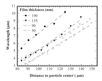
Figure 3.7 Variation of the wavelength of smooth concentric rings with the distance to the particle center for four film thicknesses (average particle diameter:  $160 \pm 29 \mu m$ )
