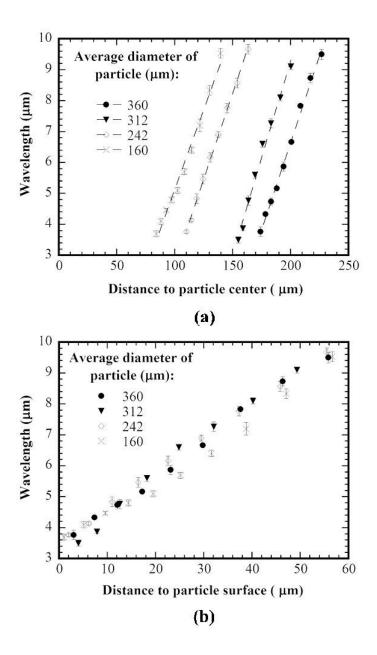
Figure 3.4 (a) Variation of the wavelength of smooth concentric rings with the distance to the particle center for four different particle sizes; (b) Variation of the wavelength of smooth concentric rings with the distance to the particle surface for four different particle sizes (film thickness: 135 nm)
