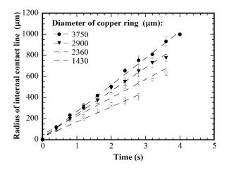
Figure 8.5 Temporal variation of the radius of the internal contact for four copper ring diameters (diameter of the copper wire: 79  $\mu$ m; film thickness: ~90 nm). The time for the onset of the internal contact line is referred to as the reference time (0s).
