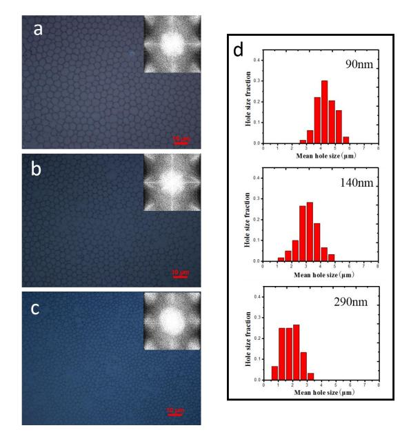
Figure 7.4 Patterns formed in zone 2 on different PMMA films; (a) ~90 nm in thickness, (b) ~140 nm in thickness and (c) ~290 nm in thickness; (d) size distribution of the holes formed on the PMMA films (surface temperature of the films at equilibrium: ~8 °C, the diameter of the copper ring is 1.45mm). Inserted images are the FFT patterns of the corresponding surface patterns.
