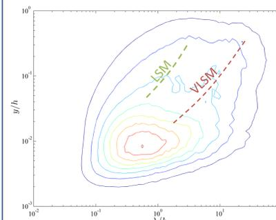
**Figure 3a:** Pre-multiplied power spectrum map for the smooth-walled case
