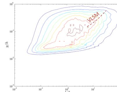
**Figure 3d:** Pre-multiplied power spectrum map for the rough-walled case: max. blowing rate
