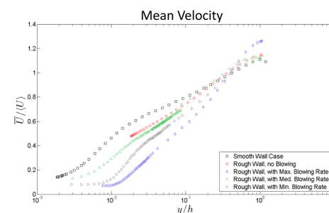
**Figure 1.** Mean velocity profiles for a range of blowing rates through the rough surface compared to the smooth-walled case with no blowing.
