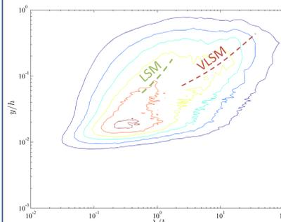
**Figure 3c:** Pre-multiplied power spectrum map for the rough-walled case: med. blowing rate
