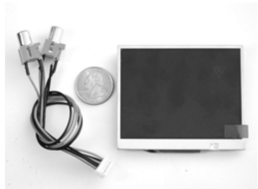
Figure 5: Jinwang 3.5" TFT Display and Driver Board
