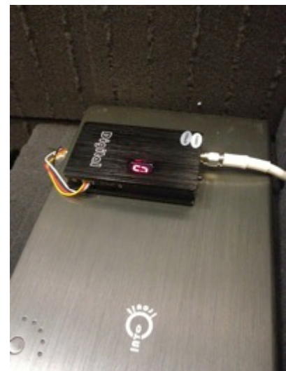
Figure 12: Mounting Location of Ground Station Video Transmitter
